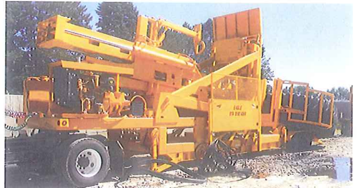
The Eagle OTR Debeader is a game-changer in downsizing the largest off-road tires and recovering their valuable rubber and steel.
